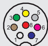
View of solder side MR8 plug (male)
